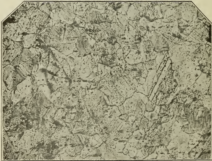
FIG. 13.—Same cylinder and same spot as Fig. 12, but after compression at 30000 lbs. per square inch. \times 200
